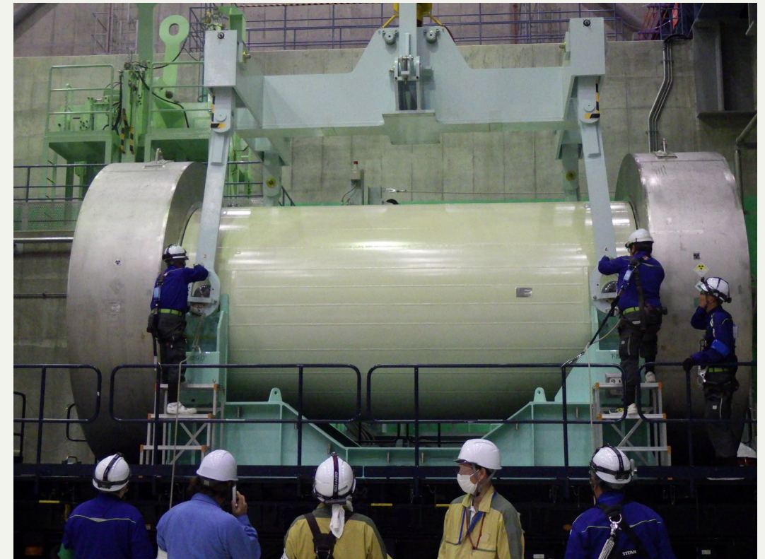
Right: Lifting the metal cask from the trailer inside the storage building (from the website of Recyclable-Fuel Storage Company)
